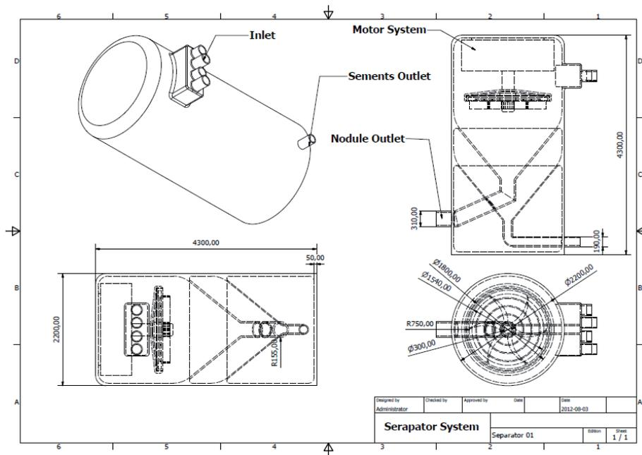
**Figure 3.20:** Design of the separation system.
