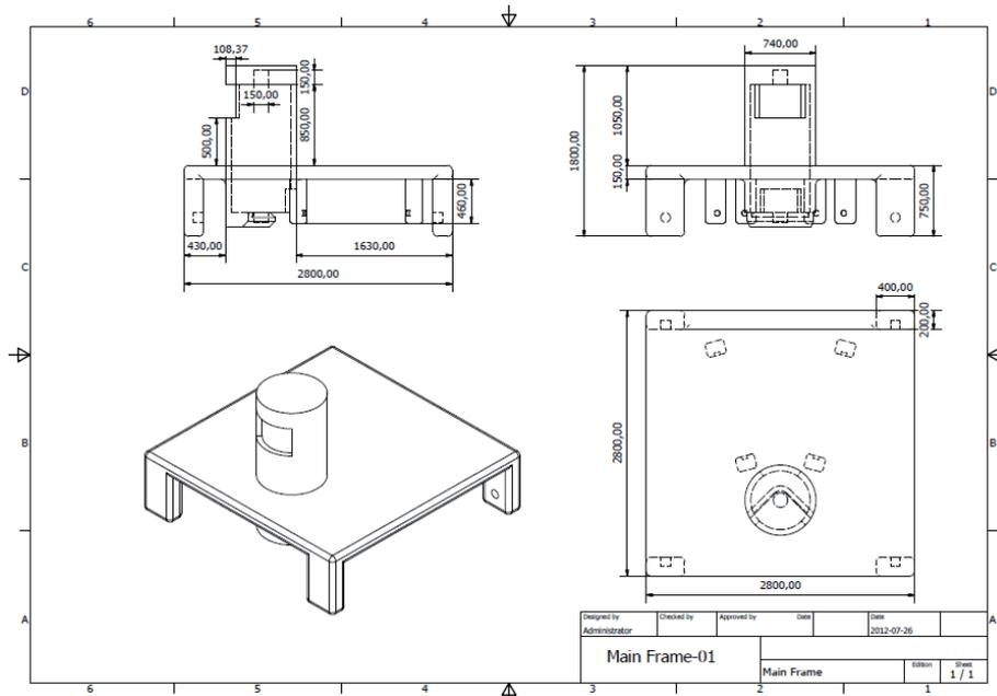
**Figure 3.13:** Design of main frame of the collector in terms of Design Phase I.
