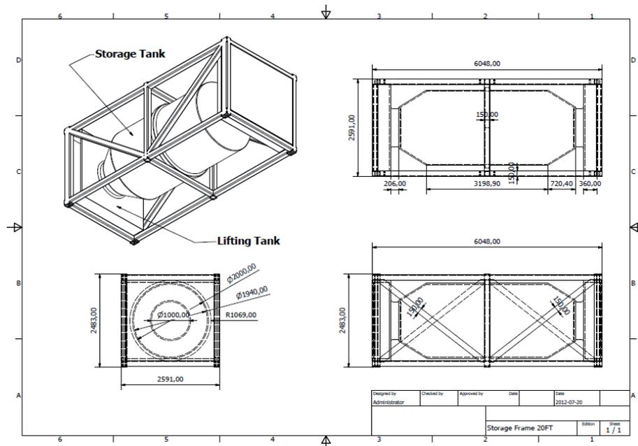
**Figure 3.22:** Conceptual drawing of the storage system, 20FT size.
