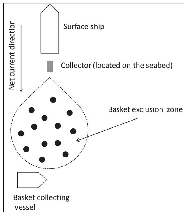
**Figure 3.41:** Top view of the proposed basket lifting system at the time of the HAZID
