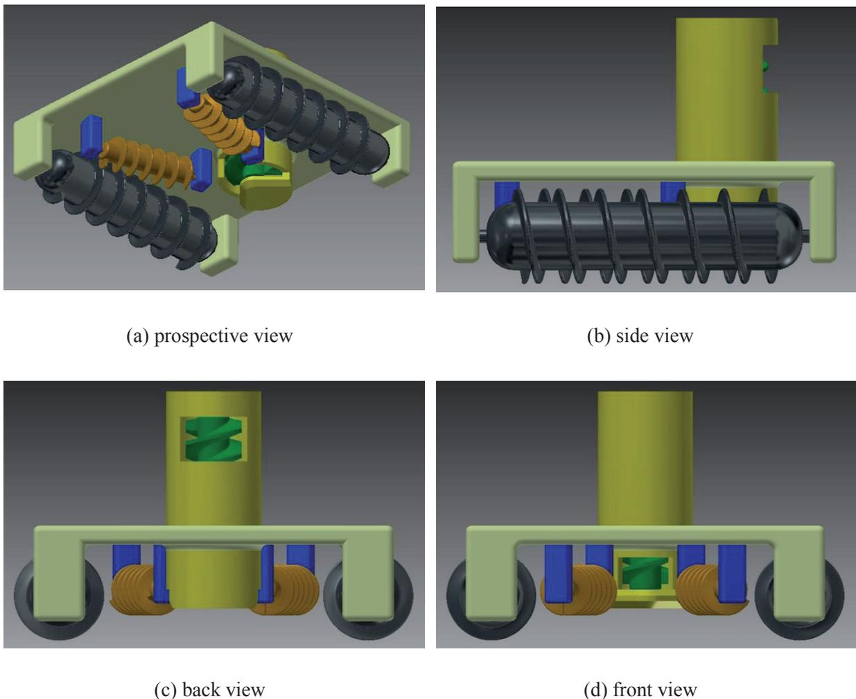
**Figure 3.5:** Conceptual design of the collector in Design Phase I.
