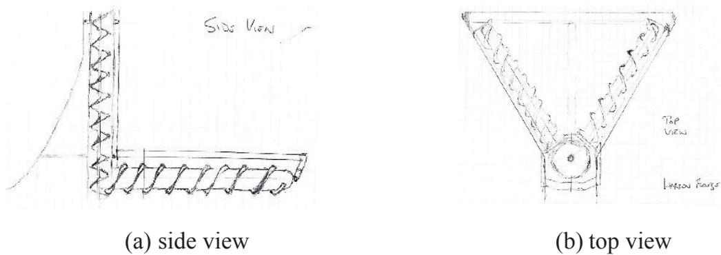
**Figure 3.4:** Hand-drawn sketch of the collector design.
