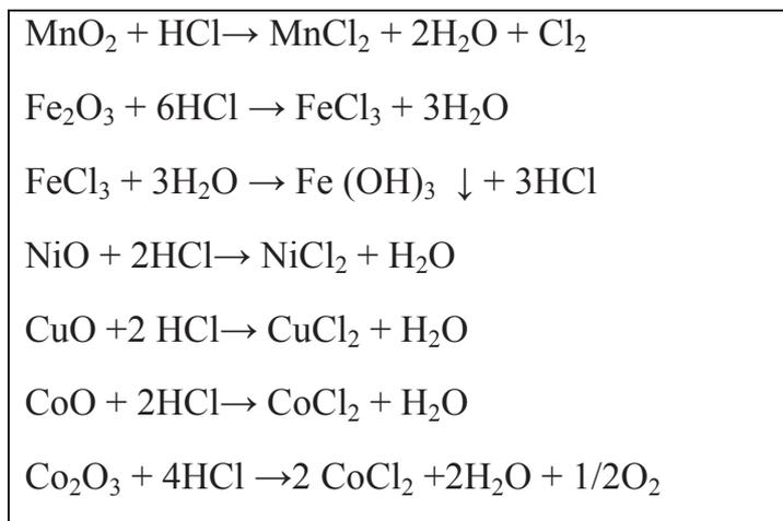
**Figure 3.32:** Typical reactions for reduction and hydrochloric acid leach (Cardwell and Kane, 1976).
