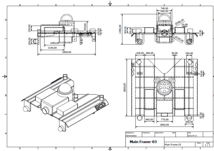
**Figure 3.15:** Design of main frame of the collector in terms of Design Phase III.
