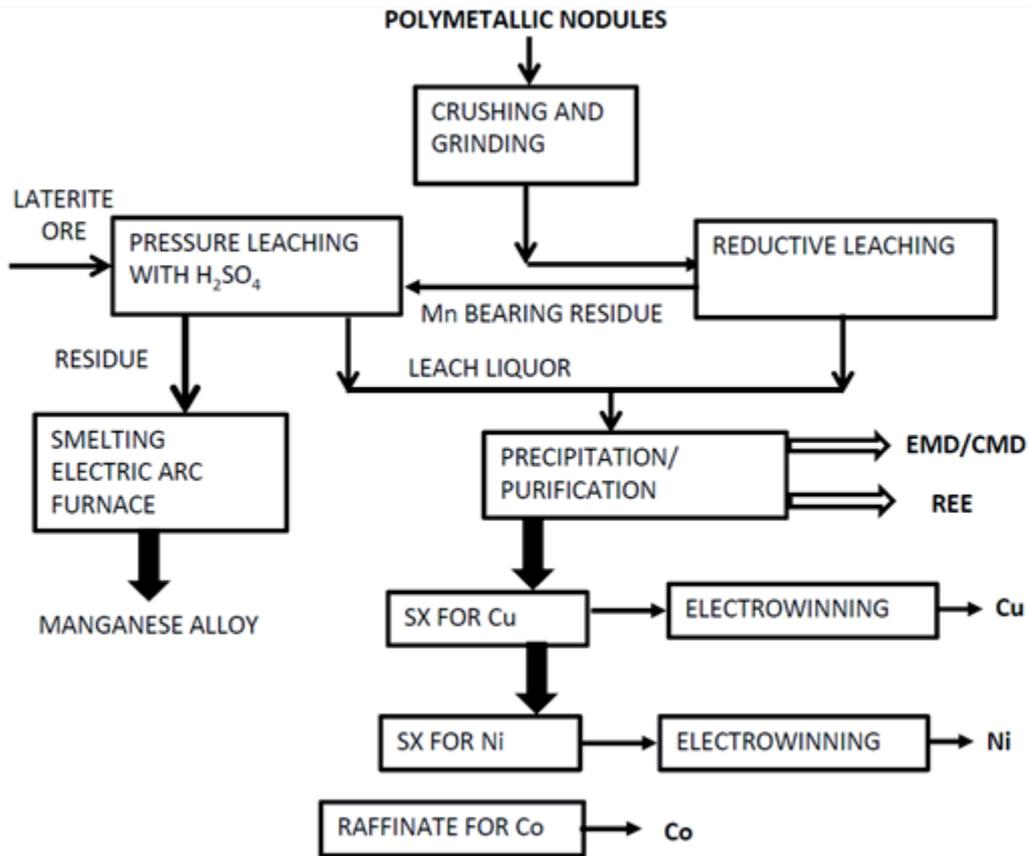
**Figure 3.35** Processing concept proposed by the Group with potential for 4-metals and Rare Earth Elements
