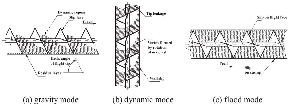
**Figure 3.2:** Classifications of the conventional screw system.
