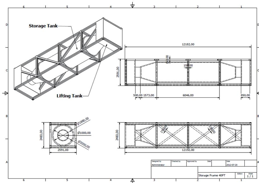
**Figure 3.24:** Conceptual drawing of the storage system, 40FT size.
